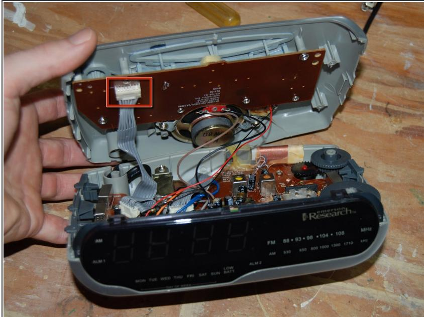
! There is a ribbon and three wires connecting lid to bottom shell.
