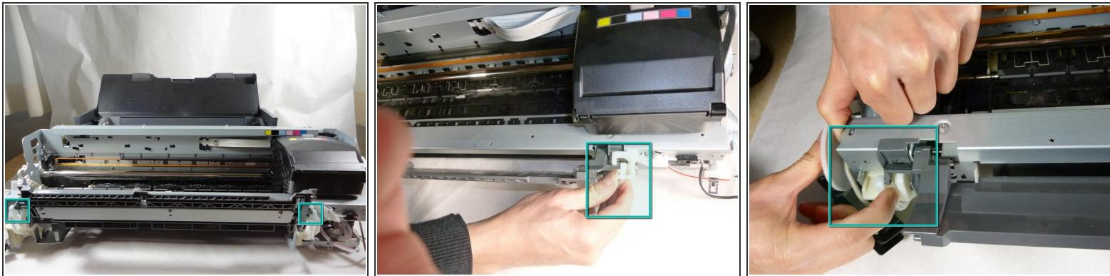
ⓘ Two guide pins secure the paper EJ assy in place.
