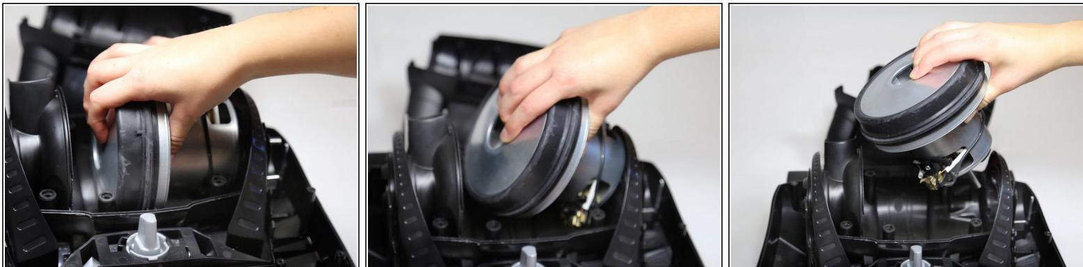
**ⓘ** There is a black wire that connects the cover to the motor. Be careful to keep this wire connected and undamaged while removing the motor.
