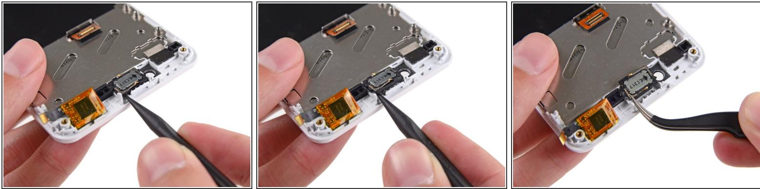
ⓘ The earpiece speaker is held to the back of the display assembly with some mild adhesive.
