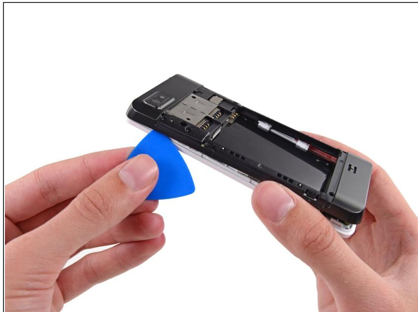
*(i)* After rounding the next corner, the midframe should be free along the bottom and the sides.
