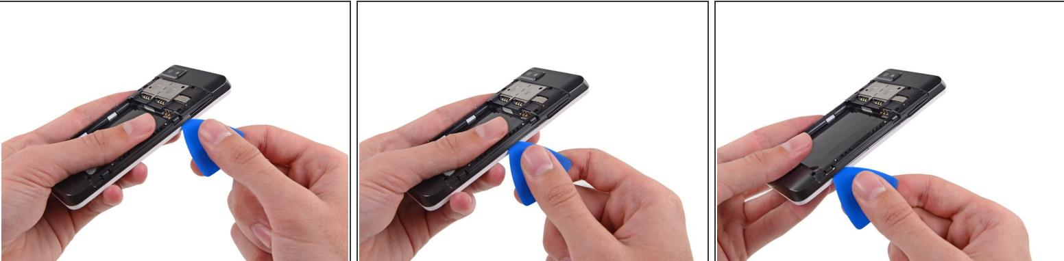
*(i)* The midframe is secured to the display assembly by several small plastic clips.
