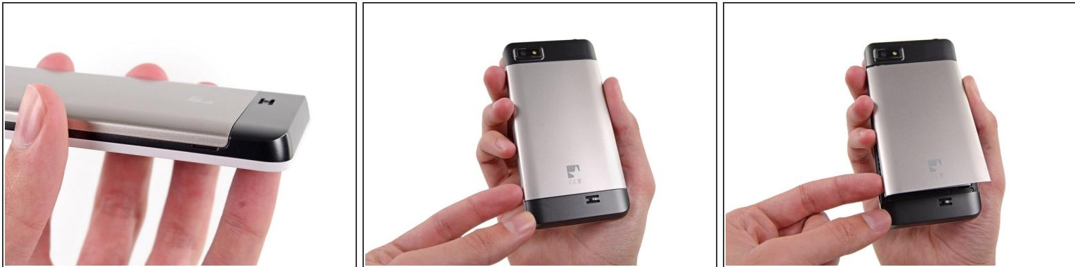
ⓘ There is a small indentation in the side of the phone near the bottom of the back cover.
