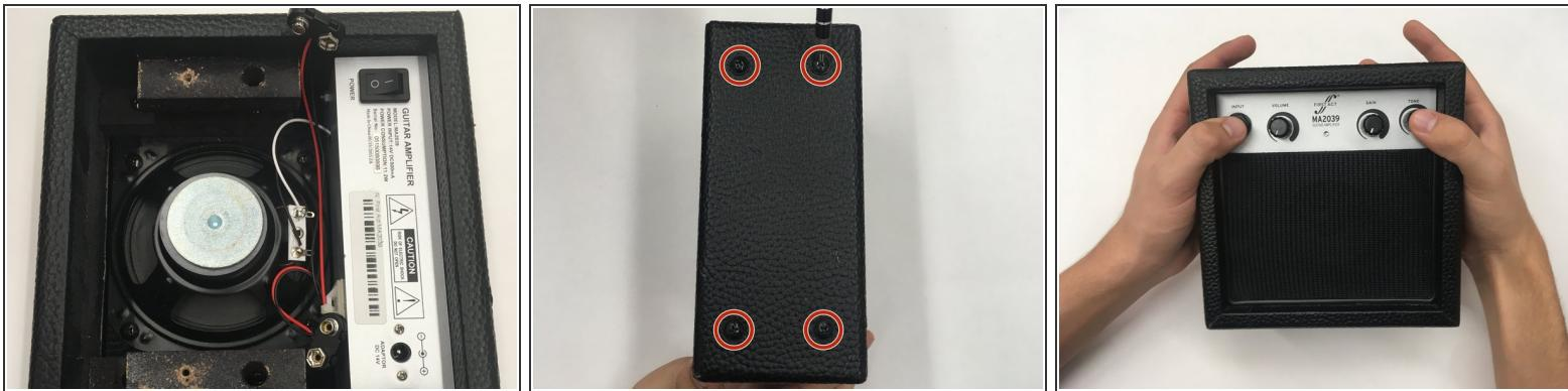
*(i)* With the back panel off, this will help make space for the silver compartment to be removed.
