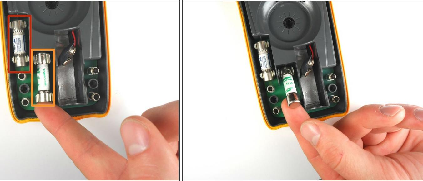
**⚠** Replace a fuse only with a fuse identical in type, voltage rating, and current rating as specified by the back panel fuse rating label or the [Fluke 77 Series III Service Manual](#). Inserting the wrong replacement fuse could create a fire hazard.
