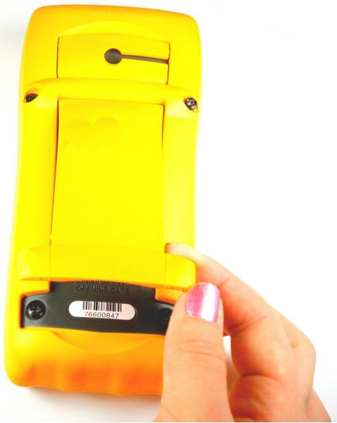
**⚠** Be sure any test leads are out and the multimeter is off before opening the device.
