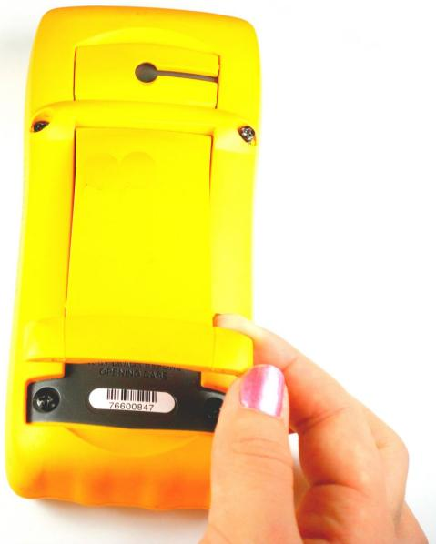
**⚠** Be sure any test leads are out and the multimeter is off before opening the device.
