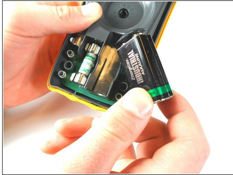
**⚠** When doing this next step, make sure to remove the battery slowly, so you don't damage the wires connecting the battery to the device.
