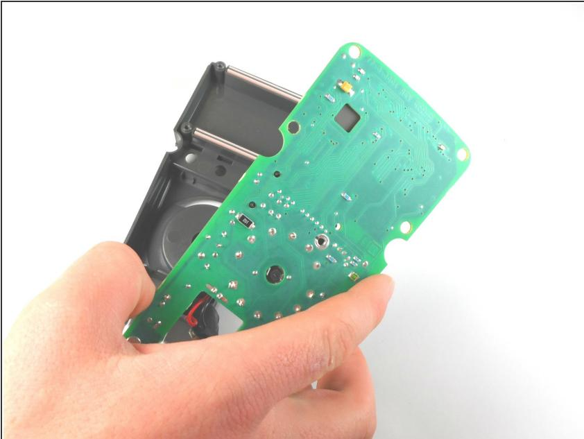
**⚠** Do not touch any of the chips on the underside of the circuit board because static electricity on your hands could damage them.
