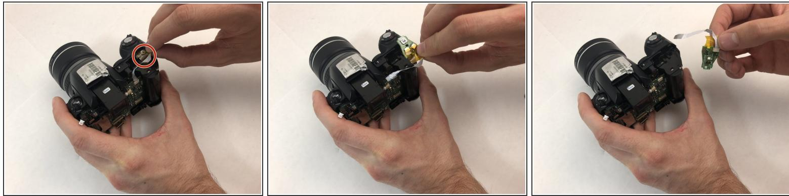
**⚠** Use caution when removing the power button chip because the opposite end of the white digital tape may be pulled out from the receiving port.
