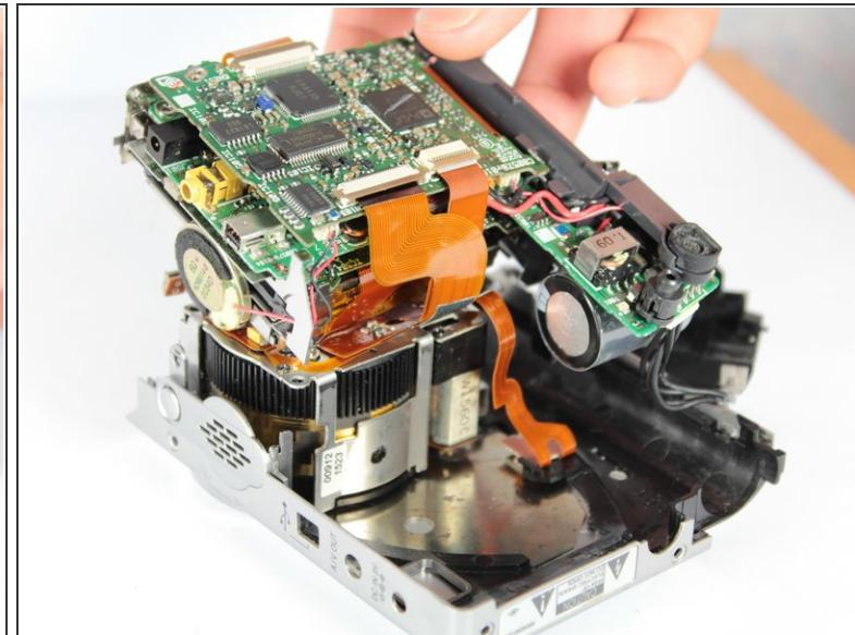
**⚠** Do not fully separate the motherboard unit from the front cover. There is still a ribbon attached and it will rip.
