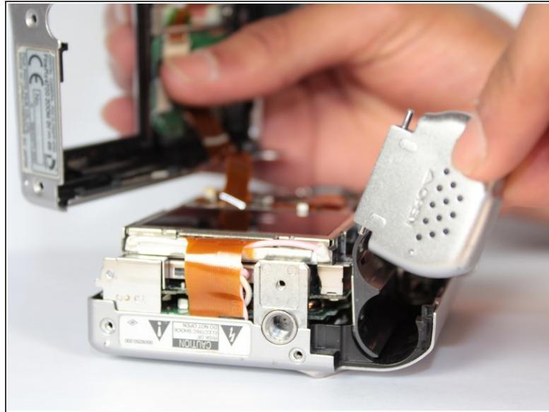
**⚠** Watch out for the orange ribbon that is still attached to the back cover when you lift it up. It is very delicate and might rip.
