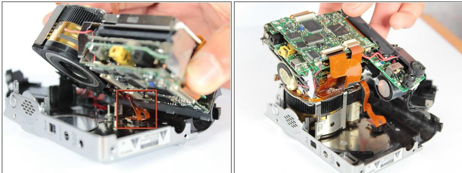
**⚠** Do not fully separate the motherboard unit from the front cover. There is still a ribbon attached and it will rip.
