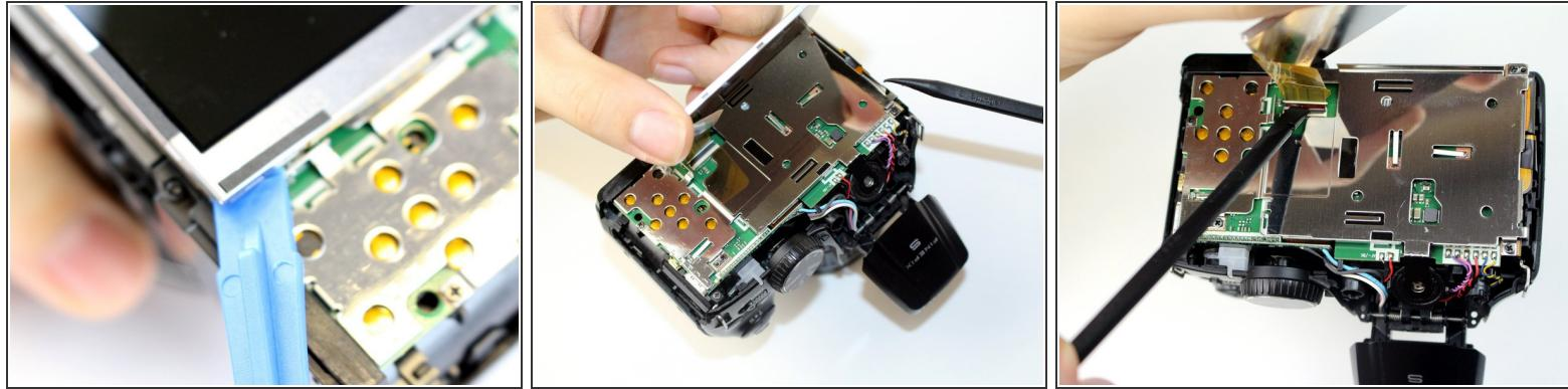
**⚠** At this point, it is highly recommended that you wear an ESD wristband to prevent damage to the internal electronic components.
