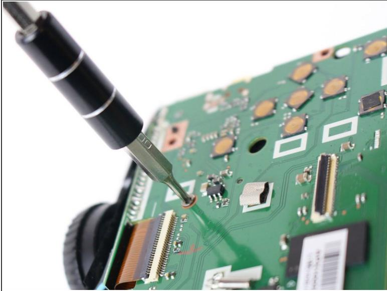
**⚠** When removing the screw attached to the motherboard, proceed slowly and apply only light pressure.
