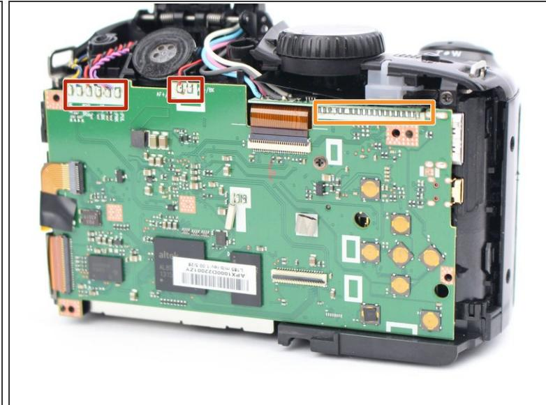
**⚠** There are two sections where wires are soldered onto the motherboard. There is also a third section where the motherboard and camera are soldered together. Please follow all safety precautions when desoldering.
