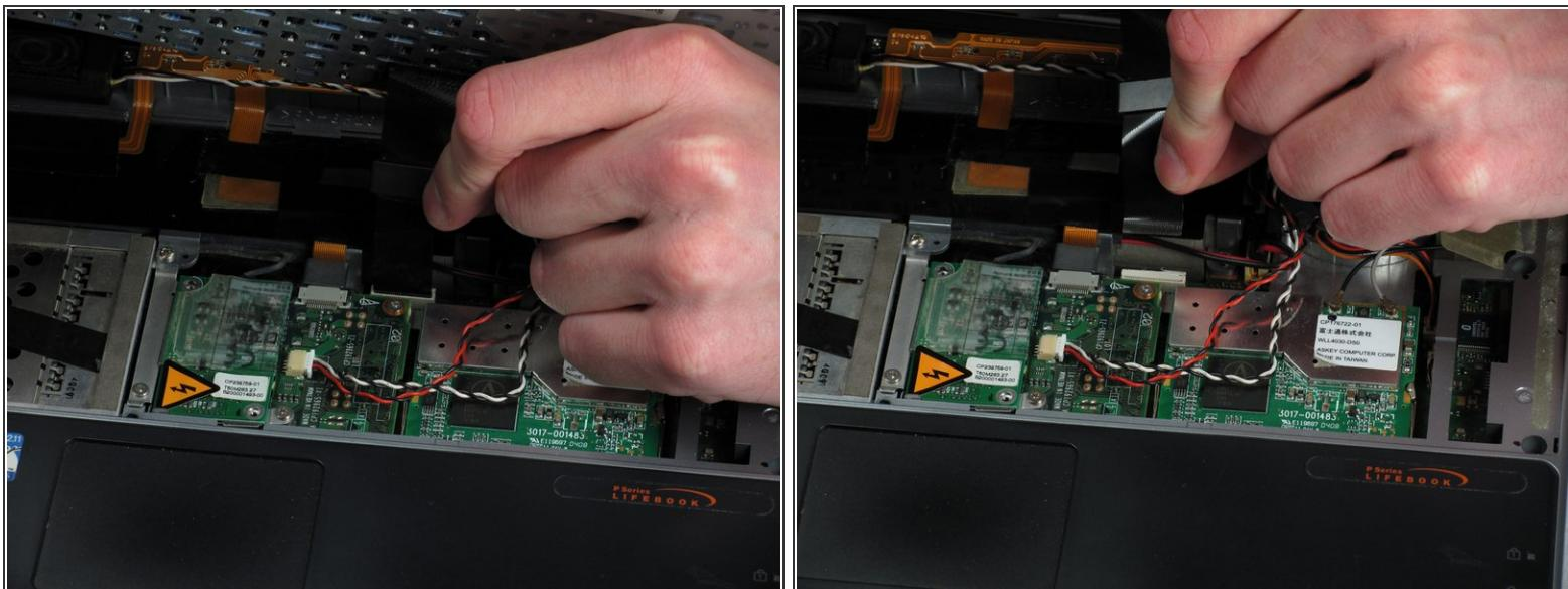
! Disconnect the keyboard by gently pulling on the hard plastic square straight up from the white connector.
