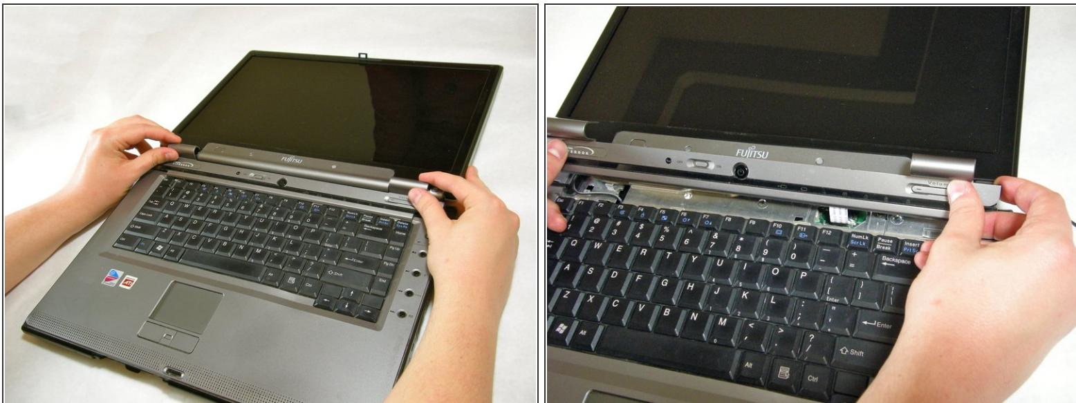
! The hinge cover has a ribbon cable that is attached to the motherboard. To prevent damage, lift the hinge cover slowly.
