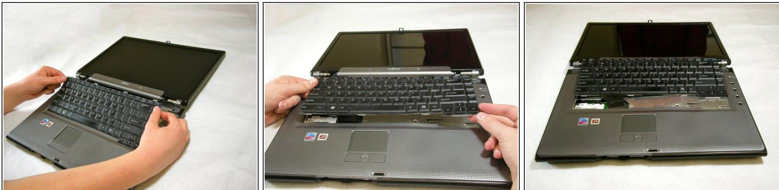
! The keyboard has a ribbon cable that is attached to the motherboard. To prevent damage, lift keyboard slowly.
