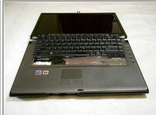
! The keyboard has a ribbon cable that is attached to the motherboard. To prevent damage, lift keyboard slowly.
