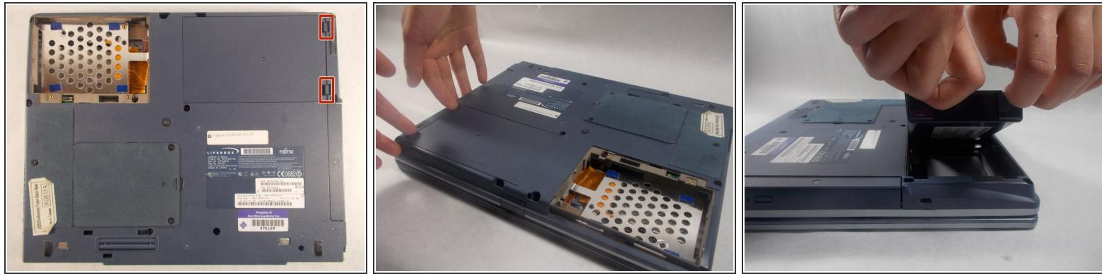
! To prevent injury, make sure the laptop is unplugged and turned off before removing the battery.
