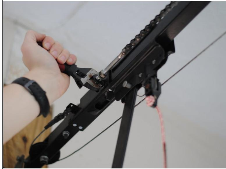
**⚠** The chain *is* under a sizeable amount of pressure. It is vital that you release that pressure safely in this step before continuing with the replacement.
