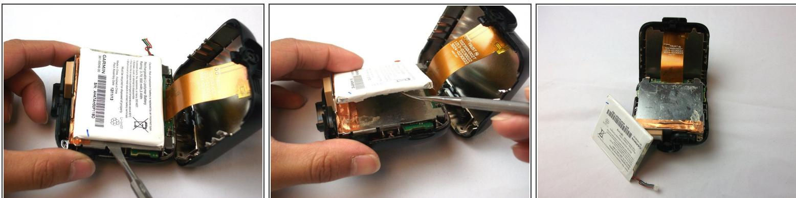
**⚠** This step shows the use of an incorrect tool. Only use ESD safe tools when handling the battery.
