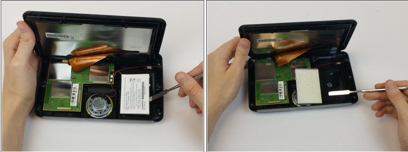
**⚠** This photo shows the use of a tool that is not ESD safe. Use a nylon spudger to complete this step.
