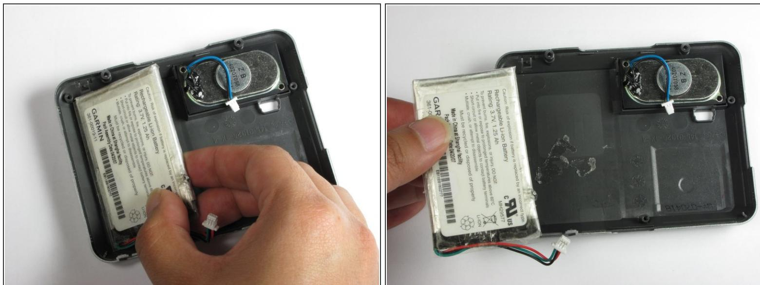
⚠ Do not use any sharp objects around the battery, as these may puncture the battery.
