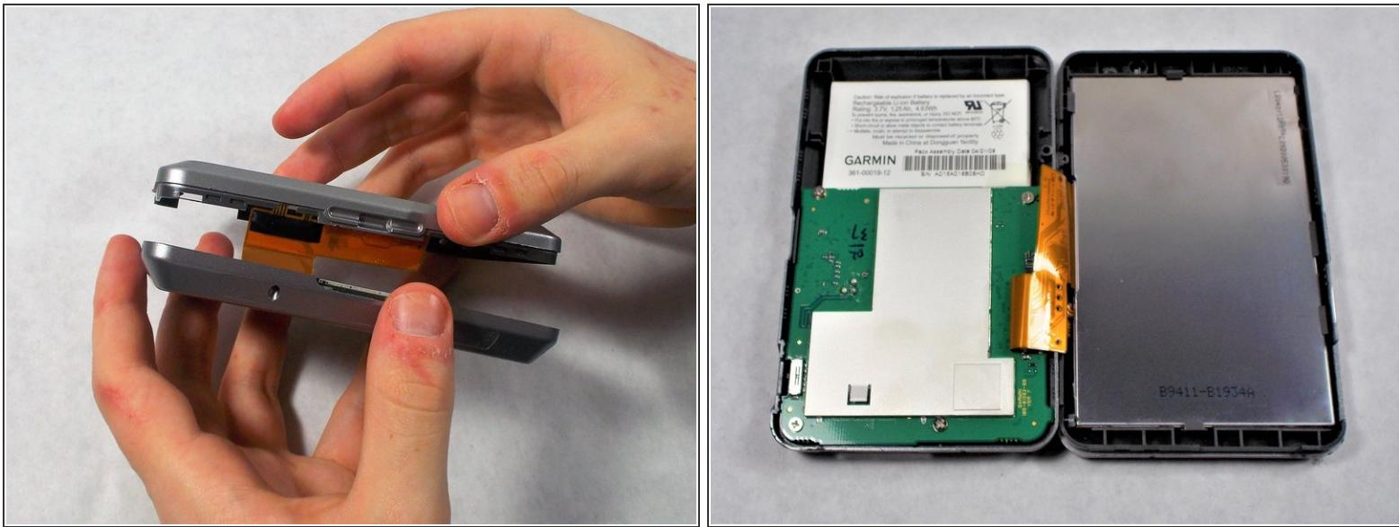
**⚠** After the case front and rear are separated, carefully lay the two sides down without disconnecting or damaging the orange ribbon cable.
