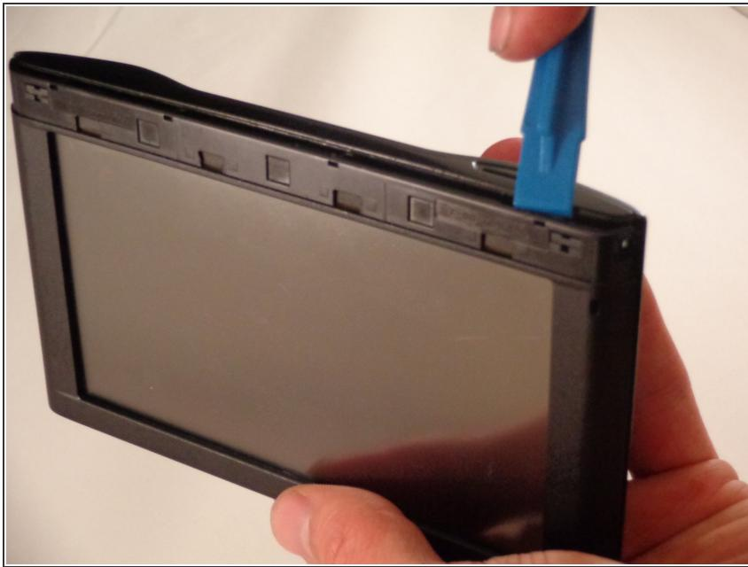
**i** There is a visible separation between the front and the back of the device.
