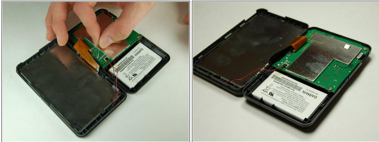
⚠ Remove the tape that is holding down the wires carefully/slowly.
