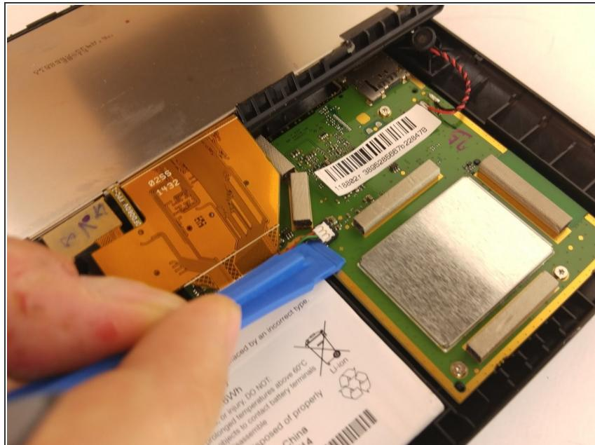
**i** The battery is connected to the main circuit board via two wires, red and green in color, and is attached with a white connector.
