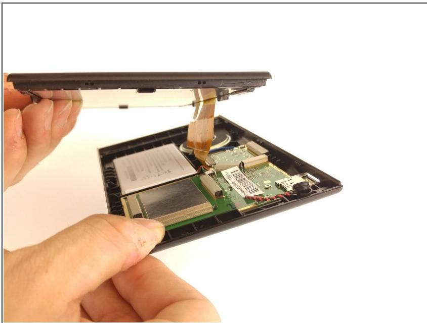
**i** Do not attempt to separate the unit until all the tabs have been separated. Once the seam is completely separated, you can lift the back away from the screen easily.
