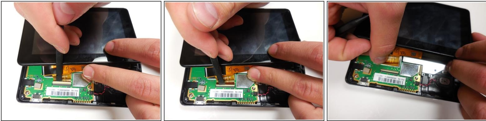
*(i)* For the larger orange connection, there is a white tab holding the connection to the circuit board.
