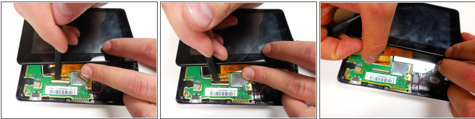
ⓘ For the larger orange connection, there is a white tab holding the connection to the circuit board.
