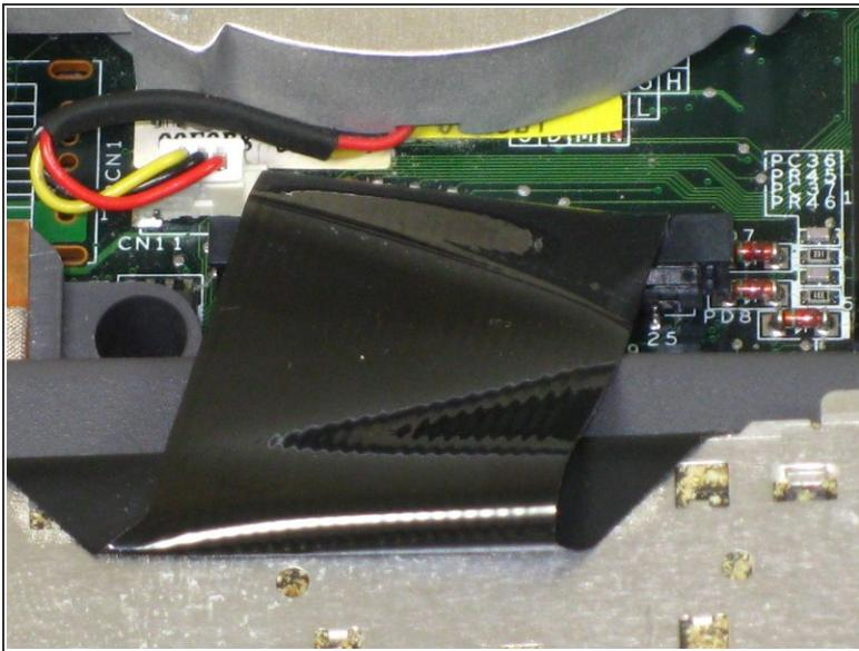
**⚠ CAUTION:** When lifting the keyboard out, do not lift keyboard up. Only fold back along the space bar edge.
