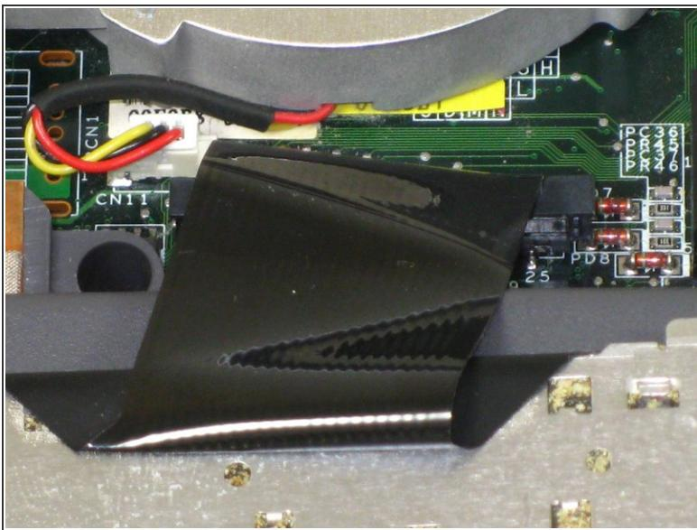
**⚠ CAUTION:** When lifting the keyboard out, do not lift keyboard up. Only fold back along the space bar edge.
