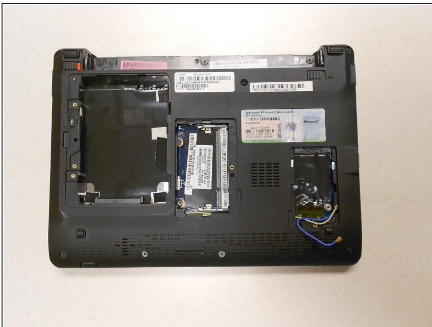
**!** Make sure the RAM, hard drive, and WiFi card have been removed from the computer before trying to take off the cover so they are not damaged in the process.
