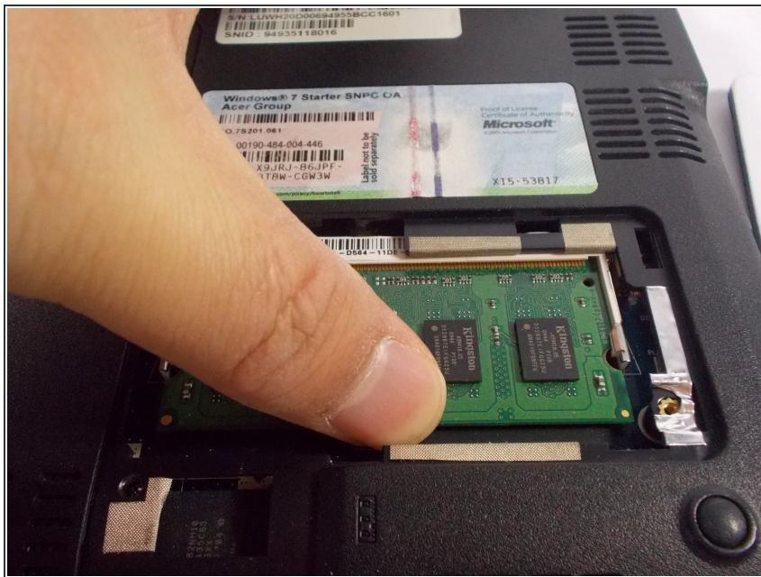
**i** When inserting the new stick of ram, be sure to insert it at the same 45° angle that the old stick of ram was taken out at. Press the stick of RAM down until it clicks into place.
