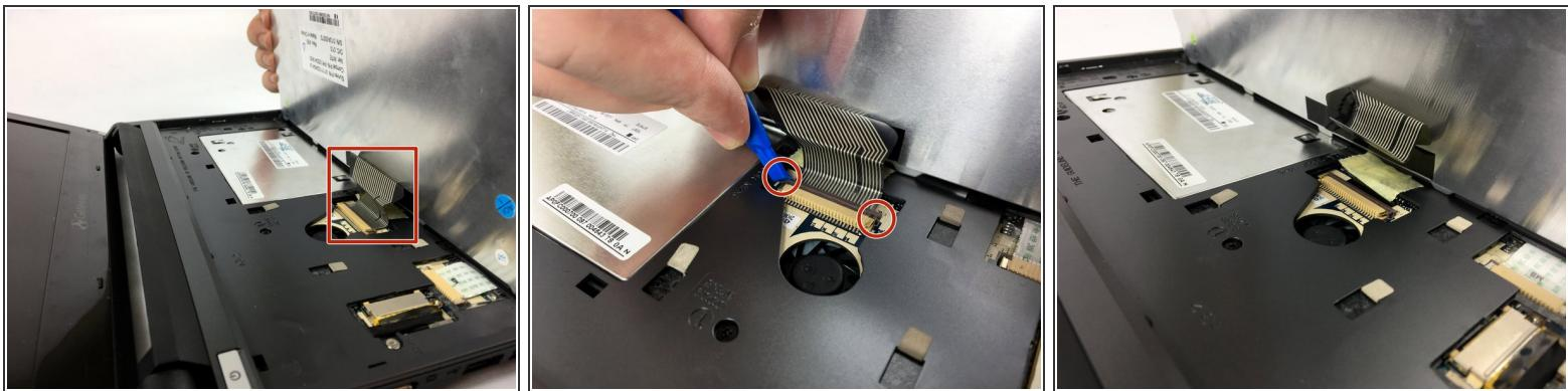
**⚠** After releasing all 5 tabs, carefully lift the keyboard along its top edge until you see the ribbon that connects the keyboard to the motherboard.
