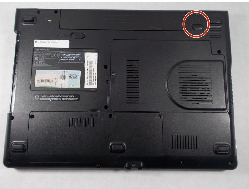
**⚠** To prevent injury, make sure the laptop is not plugged in while removing the battery!
