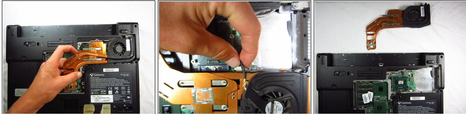
**⚠** Carefully lift up on the cooling assembly to avoid ripping the wire attaching it to the computer, and lay it upside down.
