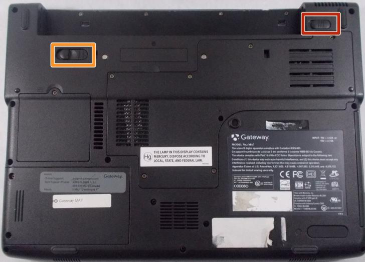
**⚠** To prevent injury, make sure the laptop is unplugged before removing the battery.
