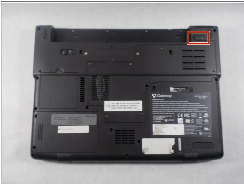
**⚠** To prevent injury, make sure the laptop is unplugged and off before removing the battery.
