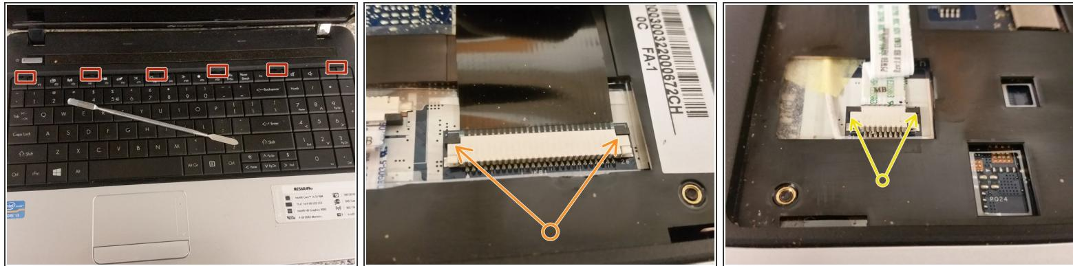
*(i)* The keyboard has no screws to remove.
