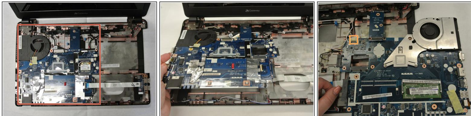
*(i)* This step requires the most caution. The CPU fan will remain attached to the motherboard.
