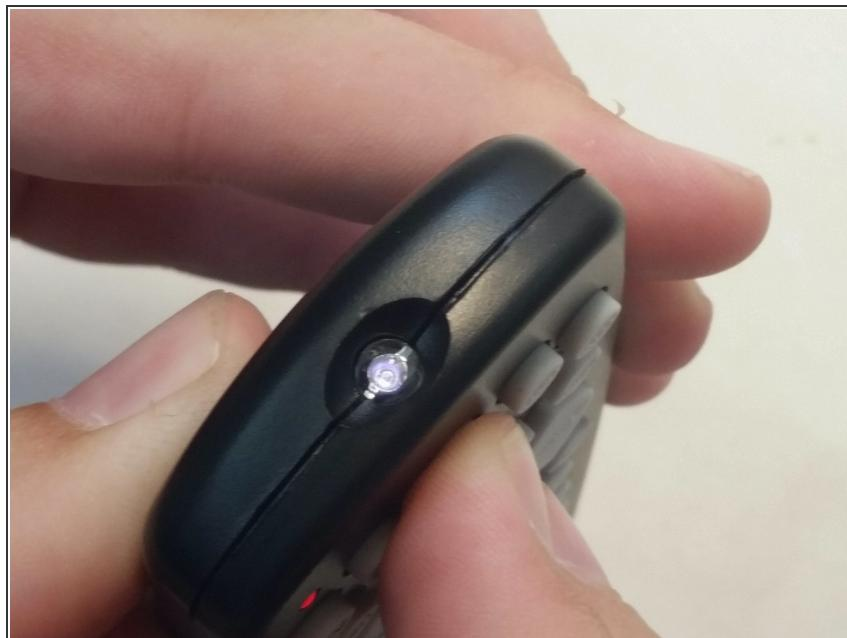
*(i)* To check if your remote is now working, check the batteries are in correctly then press a button on the remote. Aim the remote at a smartphone camera while pressing a button and you should see a flashing light being emitted.
