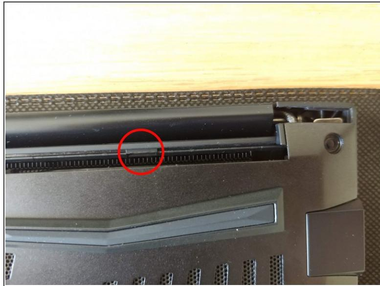
① Before removing the hood, remember that it is held by 2 aluminum rails at the back (hinge side).
