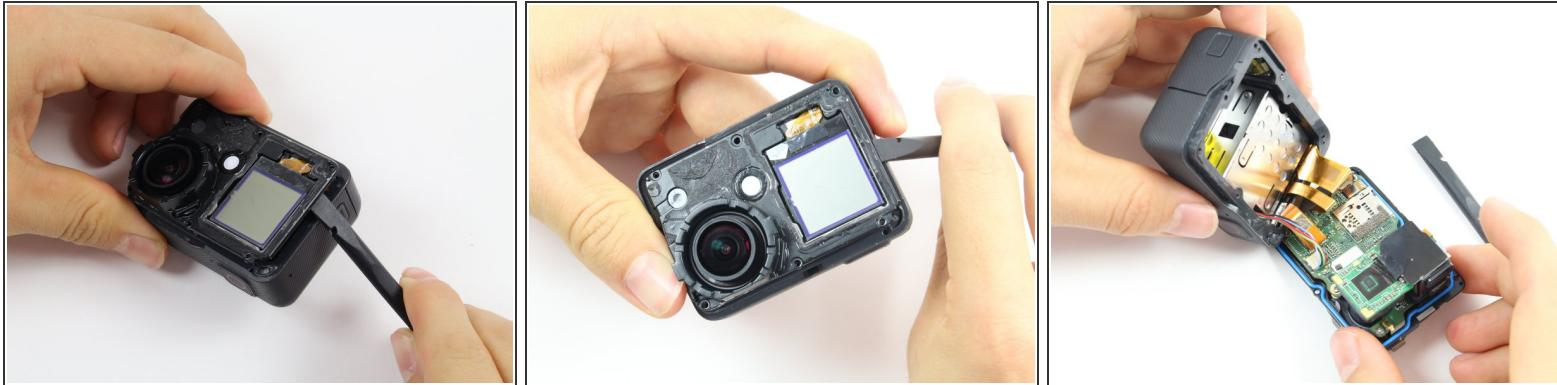
**⚠** Be careful when pulling open the motherboard assembly as it is still connected to the back housing by four cables. The cables may break if stretched.
