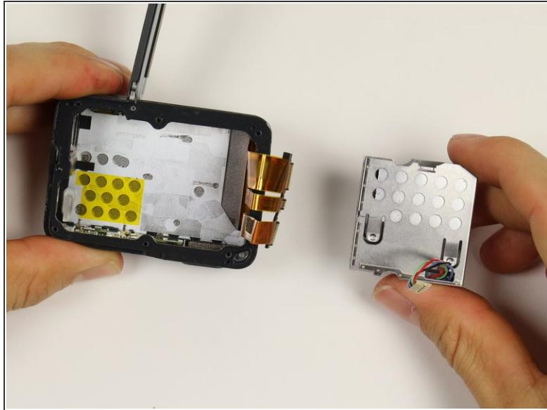
**i** Make sure the half circle grooves match up. Otherwise the battery housing will not be able to be pulled out.
