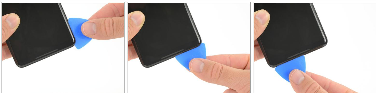
*(i)* In the following steps, use the flat edge of the opening pick, rather than a corner, to cut. This will help prevent inserting the pick too deeply.
