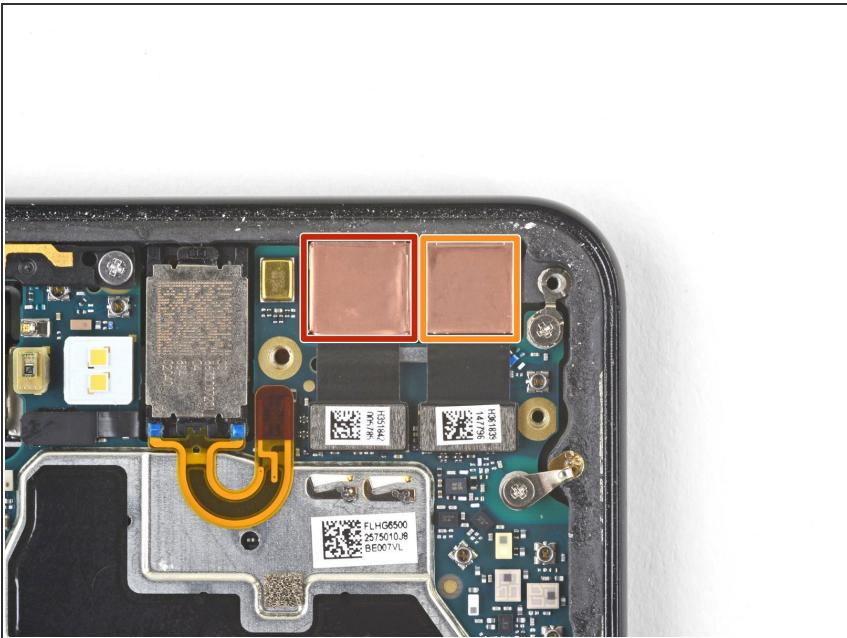
**i** If you are replacing front-facing cameras, determine which one you need to replace:
