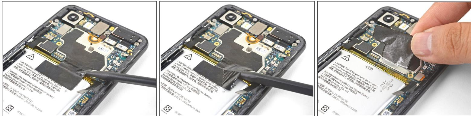
**⚠** Whenever you use the spudger near the battery, be very careful not to puncture the battery.
