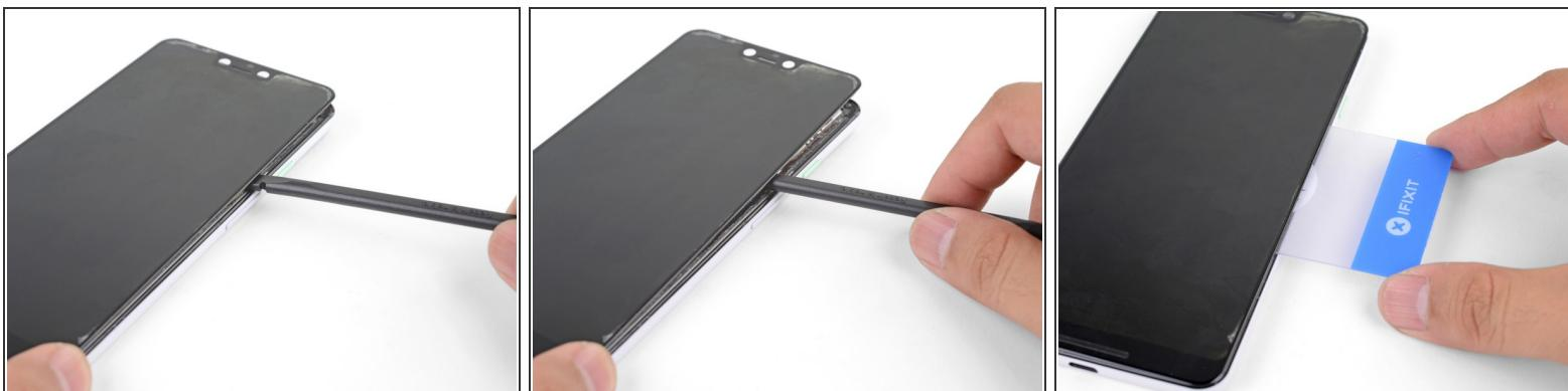
*(i)* The screen is still adhered to the frame by a large adhesive pad near the center of the screen.
